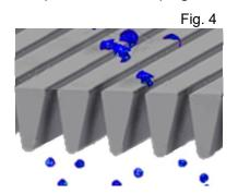
ties are retained. The wedge-shaped geometry prevents blocking on the opposite side of the wire.
